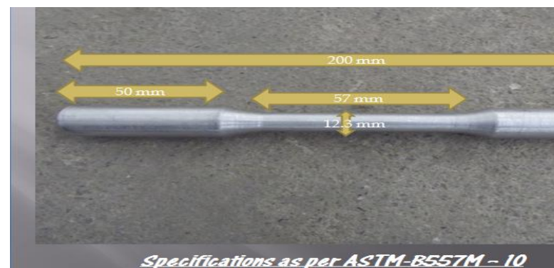
Figure 2 Dimensions of tensile specimen
