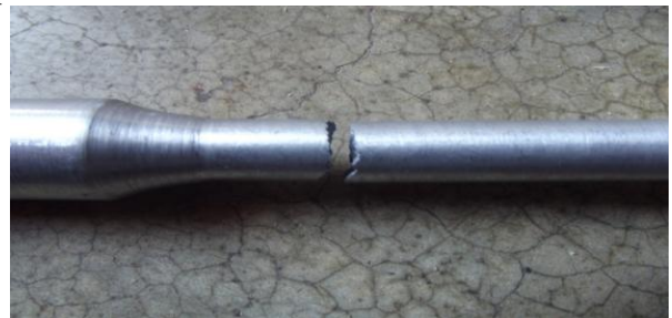
Figure 4 Photograph of the fractured tensile test specimen
