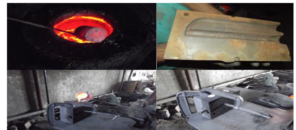
Figure 1 Die casting process used for casting the test material
